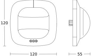
Possible mounting height: 2,50 m – 3,50 m Orange: radial and tangential
